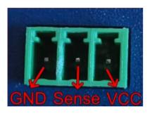
The Analog Input box is meant to be used to output a DC voltage between 5 – 24V on two pin and measure a voltage or current on the middle pin.
