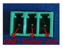
This tachometer box allow you to connect 6 sensors at the same time. The have voltage on the two outer pins and sensing on the middle pin. The box returns the frequency of the signal on the middle pin.
